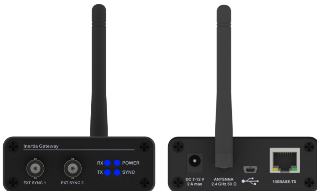
Figure 3: The front and back of the Advanced Inertia Gateway
