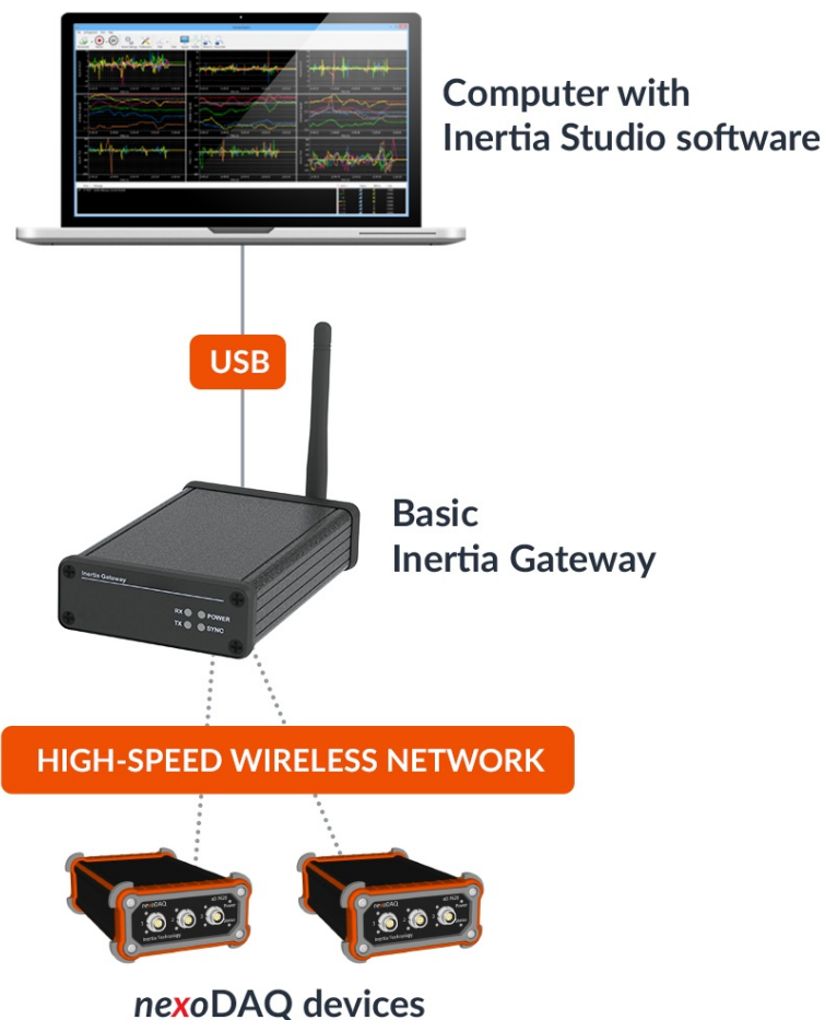
Figure 2: Typical system setup
