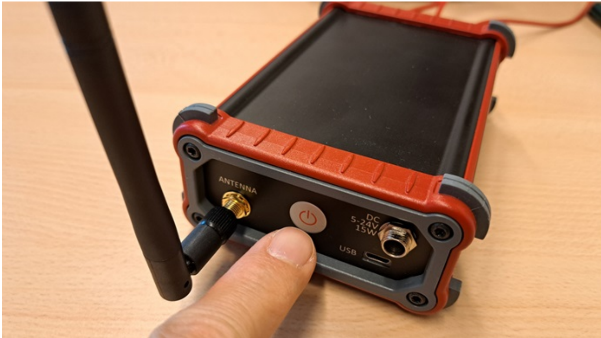
Figure 65: Power up nexoDAQ
