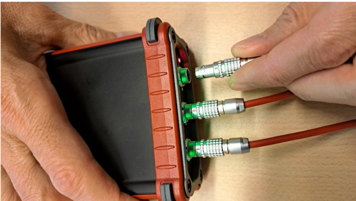
Figure 69: Connect the sensor to nexoDAQ
