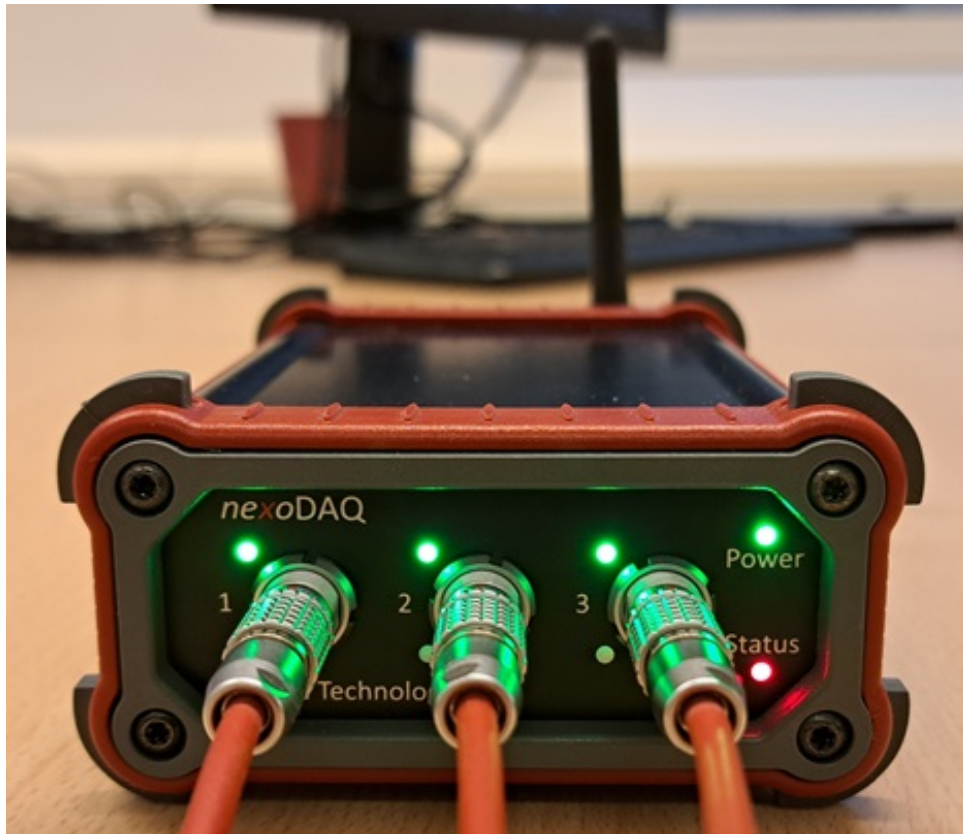
Figure 5: nexoDAQ front panel with sensors connected and wireless communication
