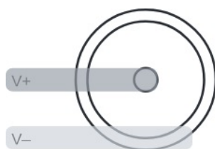
Figure 8: The barrel connector for external power supply
