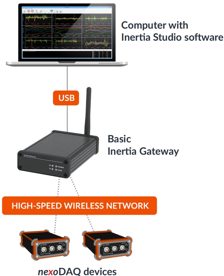
Figure 2: Typical system setup
