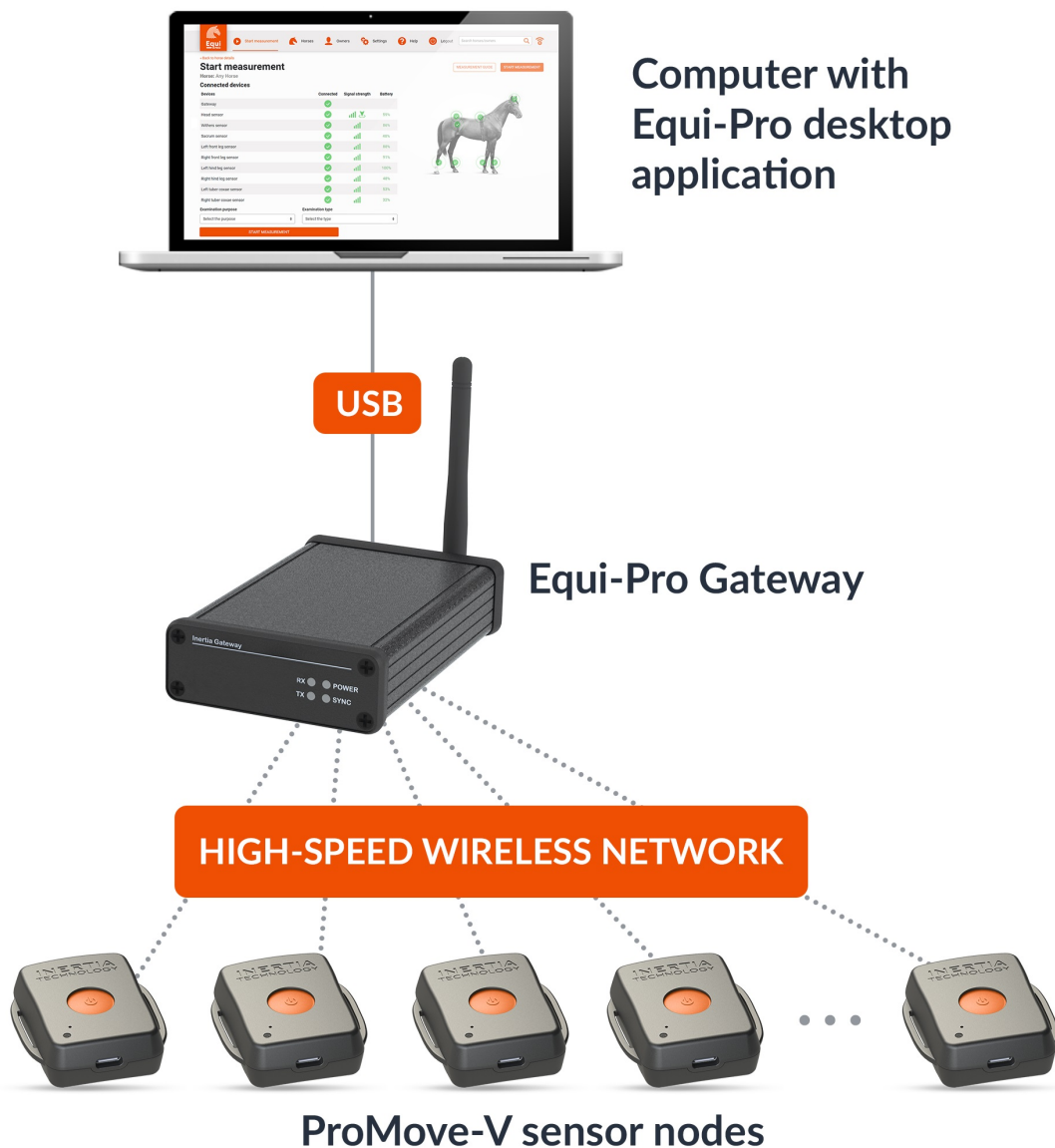
Figure 1: Equi-Pro hardware overview
