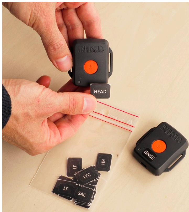
Figure 12: Placing labels on sensors depending on their position.
