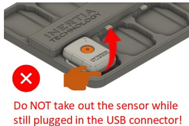
Figure 29: Incorrect removal of a sensor from the charging cradle.
