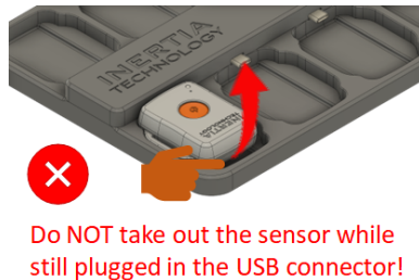
Figure 11: Incorrect removal of a ProMove-V sensor node from the charging cradle.
