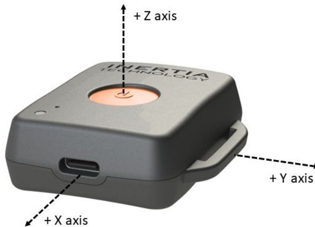
Figure 12: The ProMove-V node and the reference X, Y and Z-axis
