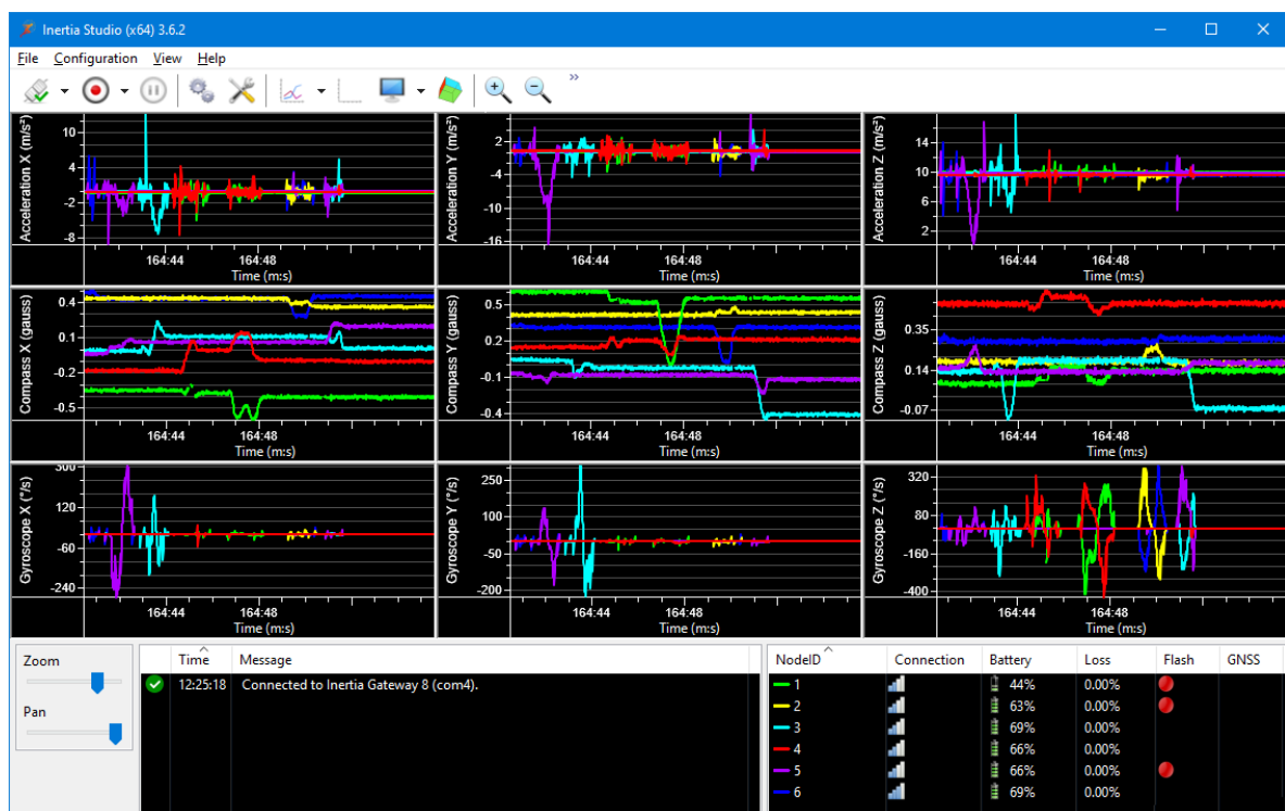
Figure 15: Inertia Studio with six nodes, showing data from the accelerometer, compass and gyroscope
