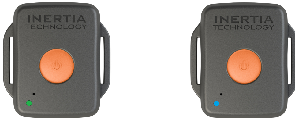
Figure 3: The ProMove-V node top view with green and blue LEDs
