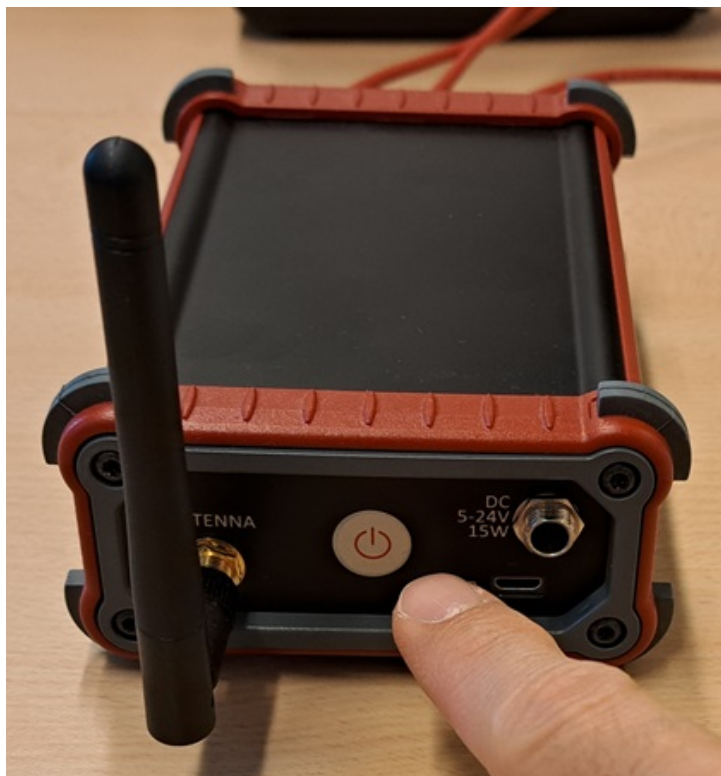
Figure 7: nexoDAQ back panel with power, micro-USB and antenna connectors, and the power button
