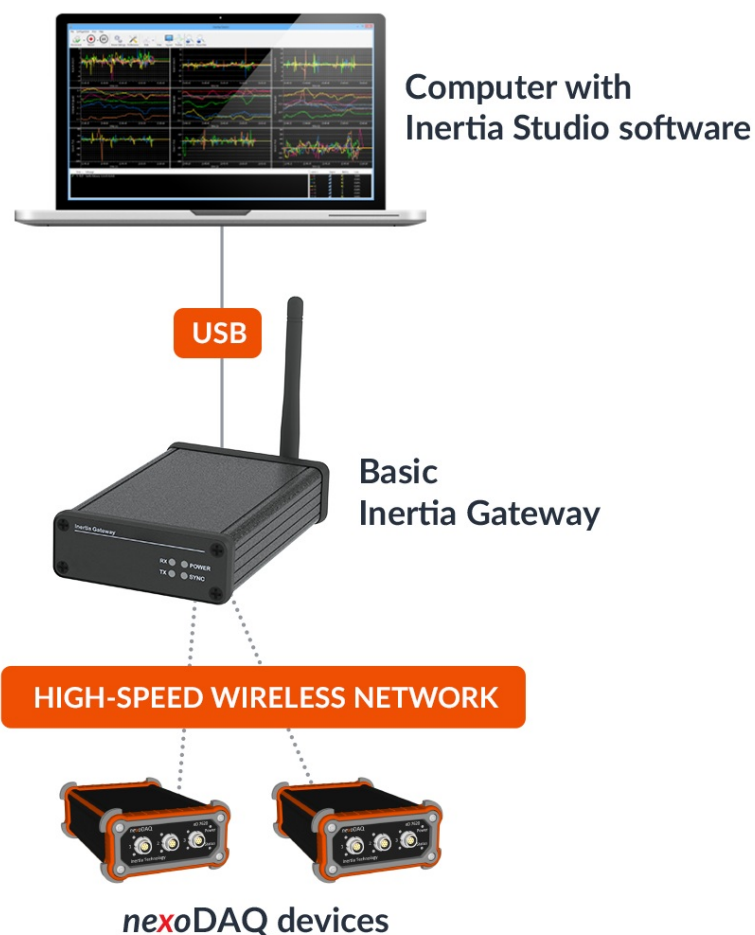
Figure 2: Typical system setup
