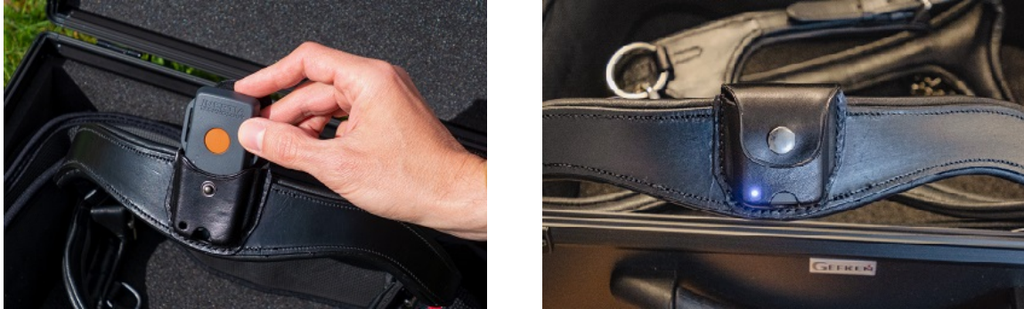
Figure 14: Inserting the head sensor in the pocket of the bridle.
