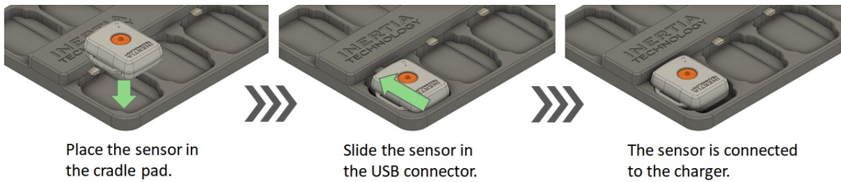
Figure 27: Inserting a sensor into the charging cradle.
