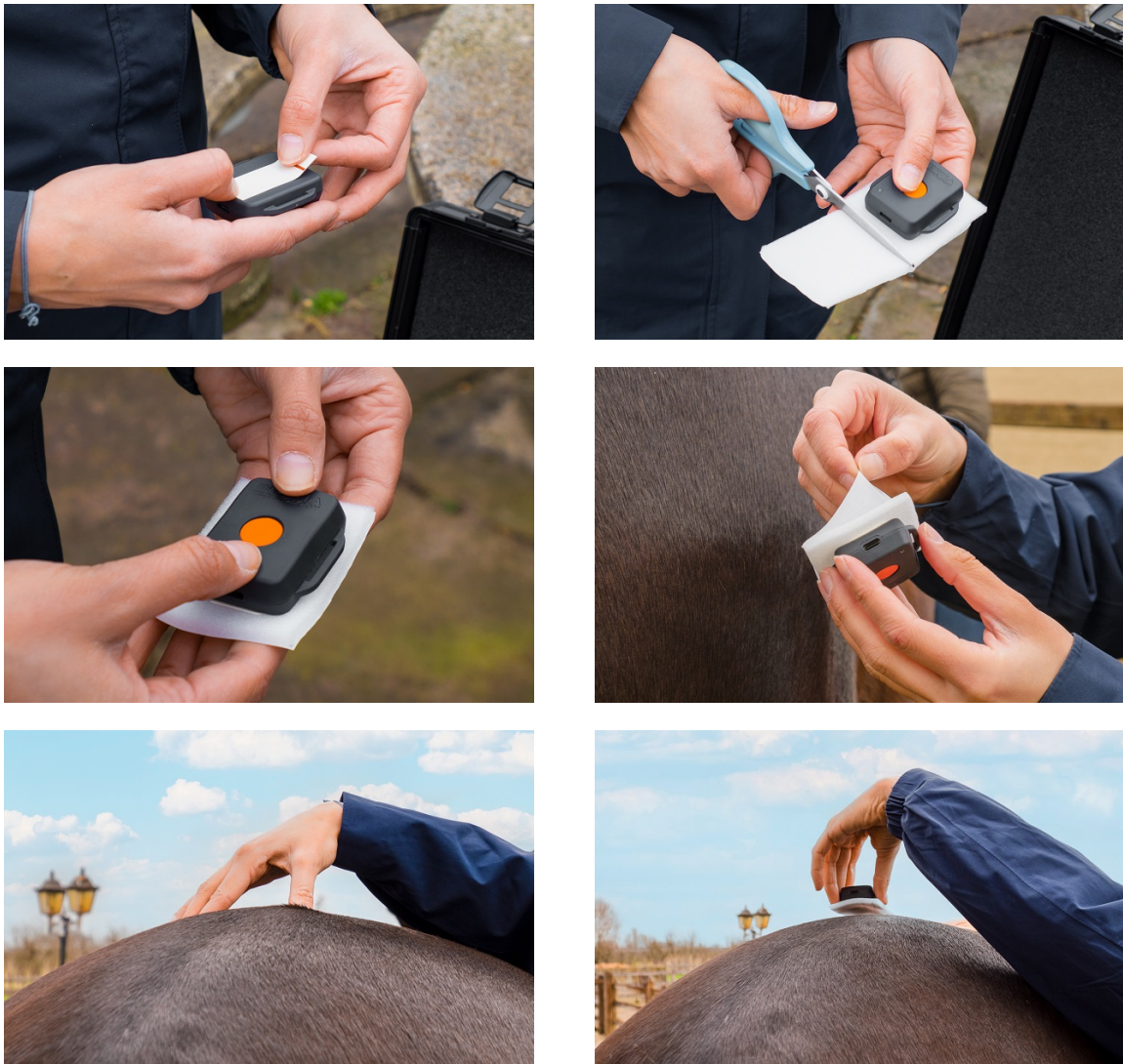
Figure 18: Attaching the sacrum sensor
