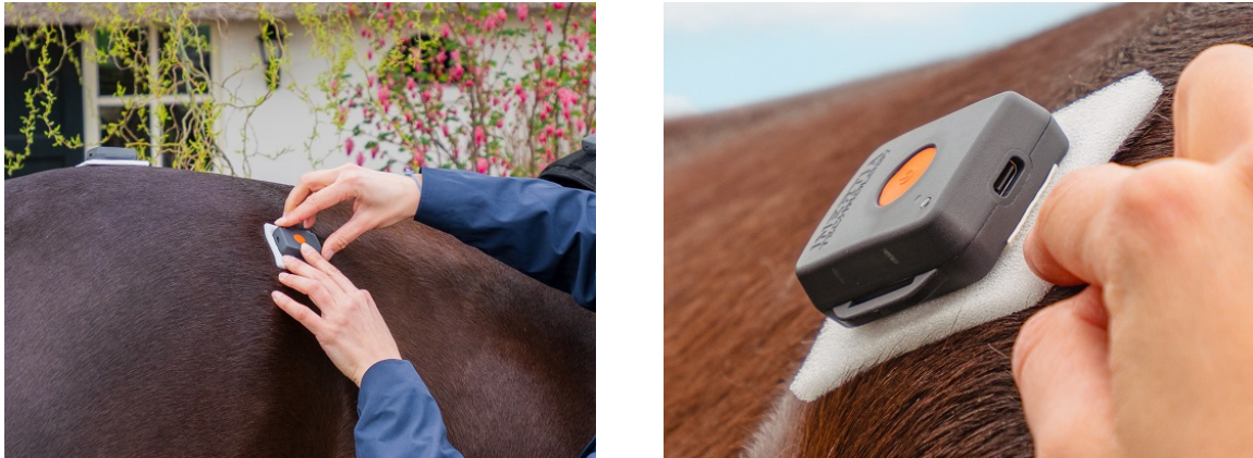
Figure 19: Attaching the RTC and LTC sensors
