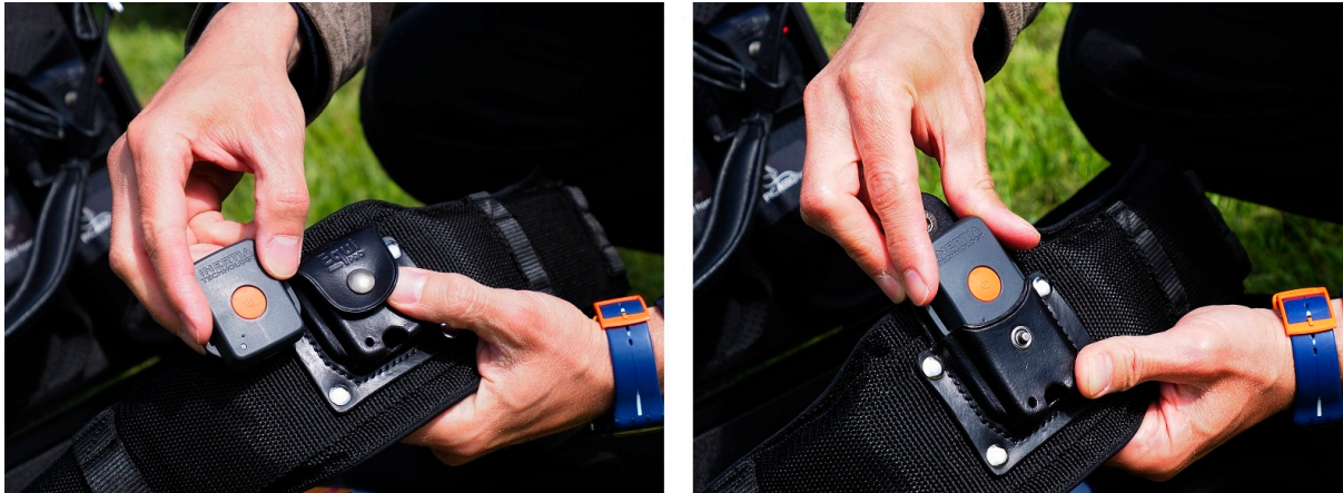
Figure 16: Insert the withers sensor in the girth pocket.
