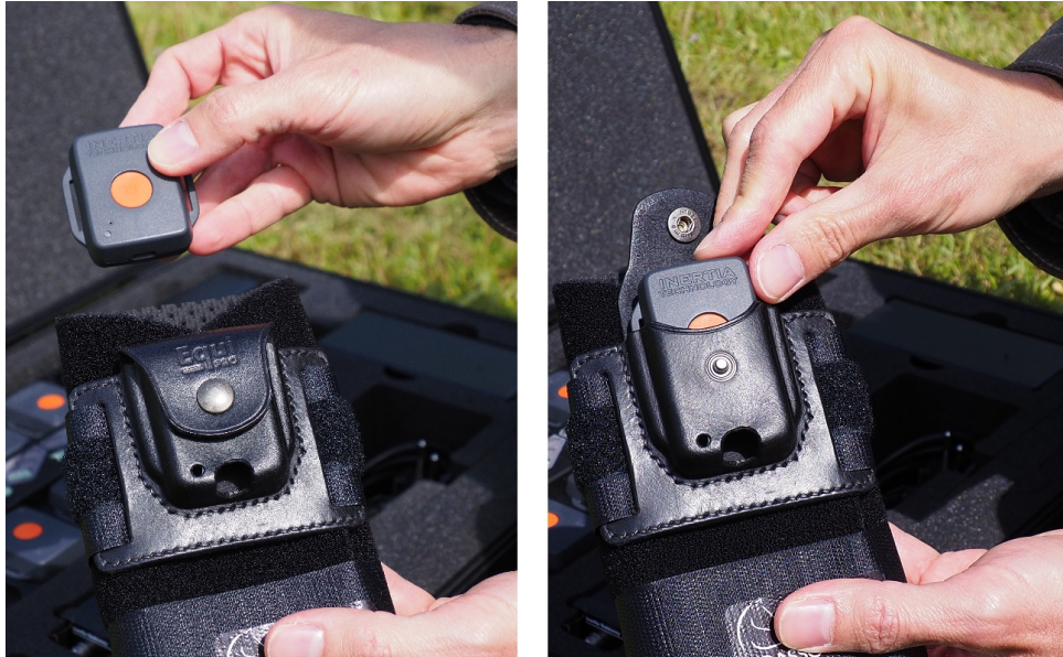
Figure 20: Inserting sensors in the leg pocket
